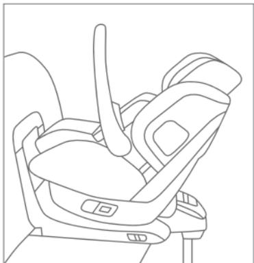
**Important:** The coloured indicators on the side of the infant carrier must switch from red to green. Your child may already be placed and secured into the seat while doing this. Once the carrier is locked into place, rotate the child seat into the rearfacing position.
