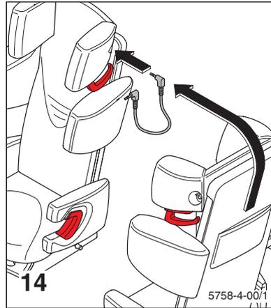
Remove the loudspeaker cable from the pocket on the back of the child seat.
