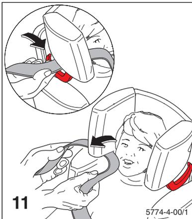
**2. Correct positioning of the lap belt**
